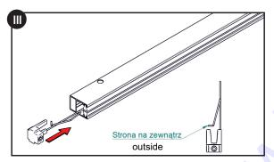
3.Insert the KLIK-KLAK clip into the guides from the bottom, paying attention to placing them in the correct guide.
