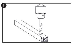
Drill holes in the guides approx. 2" away from the top and bottom edges and at intervals of 10-20" between holes.
