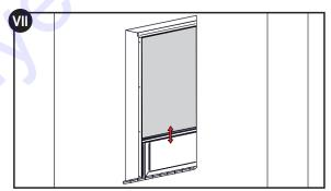
7.Check the correct functioning of the mosquito net. If necessary, change the height of the attachment of the catches in the guides.
