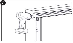
Place the mosquito net on the window and screw it to the window frame after checking the vertical and level.
