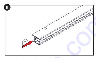
2.Insert the bottom plugs into the guides.
